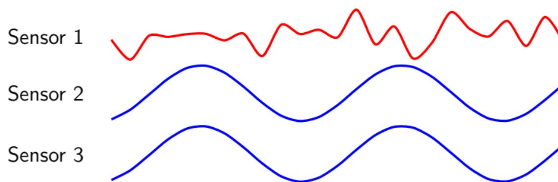
By inspection of the signals, easy to tell that Sensor 1 has been corrupted.
