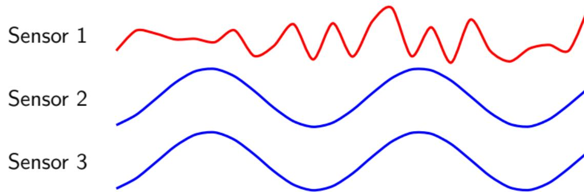
Suppose there are 3 sensors measuring the same system. We know the *number* of sensors which have been corrupted, but not which ones.
