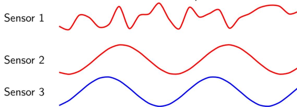
Suppose there are 3 sensors measuring the same system. We know the *number* of sensors which have been corrupted, but not which ones.
